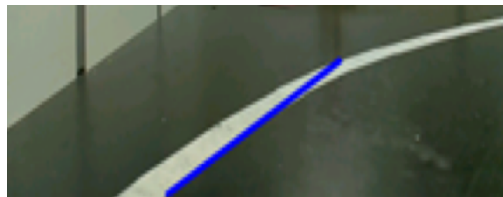
Detecting only the left lane marking in a right-hand turn
