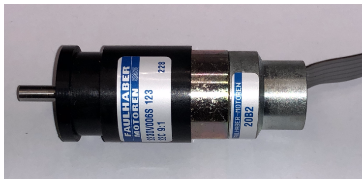
Figure 1.4: Incremental encoder (left); motor with encapsulated gearbox and encoder (right)
