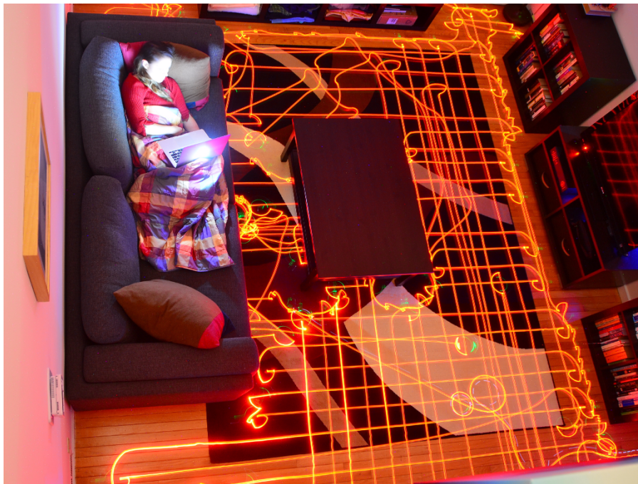
Figure 3.2: Roomba 980 cleaning pattern [Ackerman 2016] Photo courtesy of Evan Ackerman / IEEE Spectrum 2016
