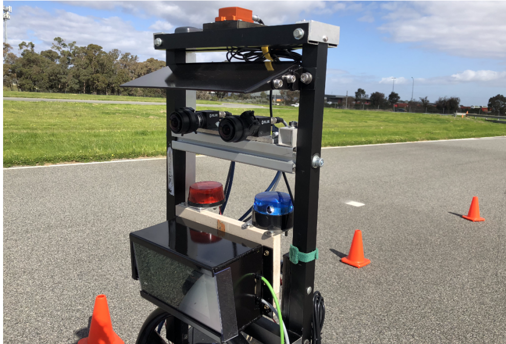
Figure 14.3: Sensor stack on top of REV car: IMU, stereo cameras, Lidar
